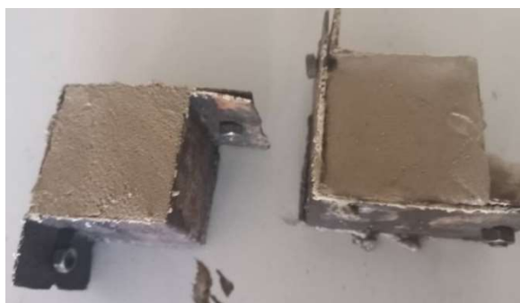
Figure 1: Rammed refractory bricks.
