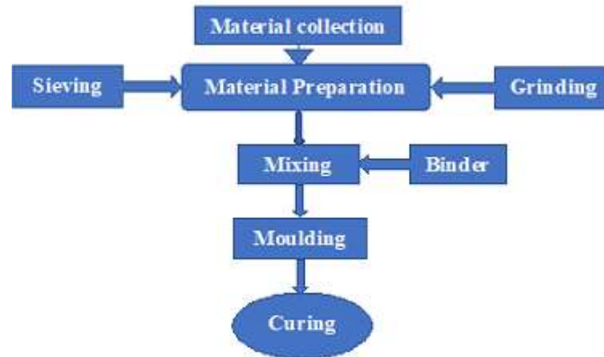
Figure 3: Brake pad liner production flowchart.
