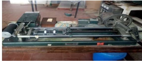
Figure 6: Monsanto testing machine for hardness and shearing.
