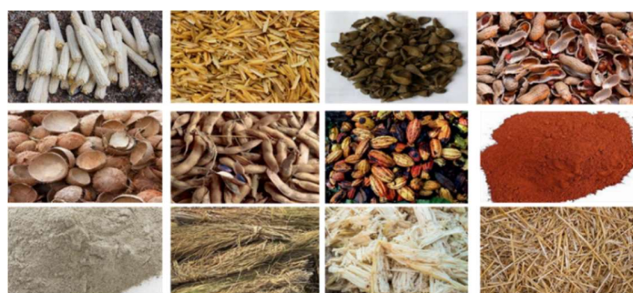
Figure 4: Agricultural and industrial wastes used as reinforcement in AMMC development.
