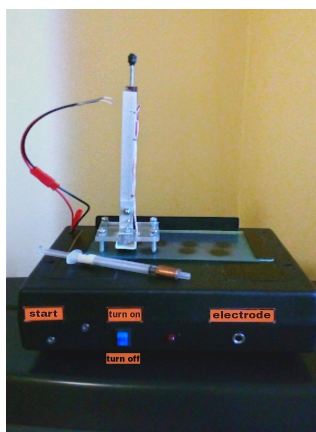
Figure 1: Device for researching CGD with H 2 O drops.
