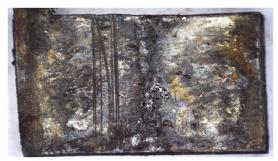
Figure 4: Effect of HCl solution on TS (without CP, and after corrosion).
