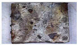
Figure 5: Effect of the H<sub>2</sub>SO<sub>4</sub> solution on TS (without CP and after corrosion).
