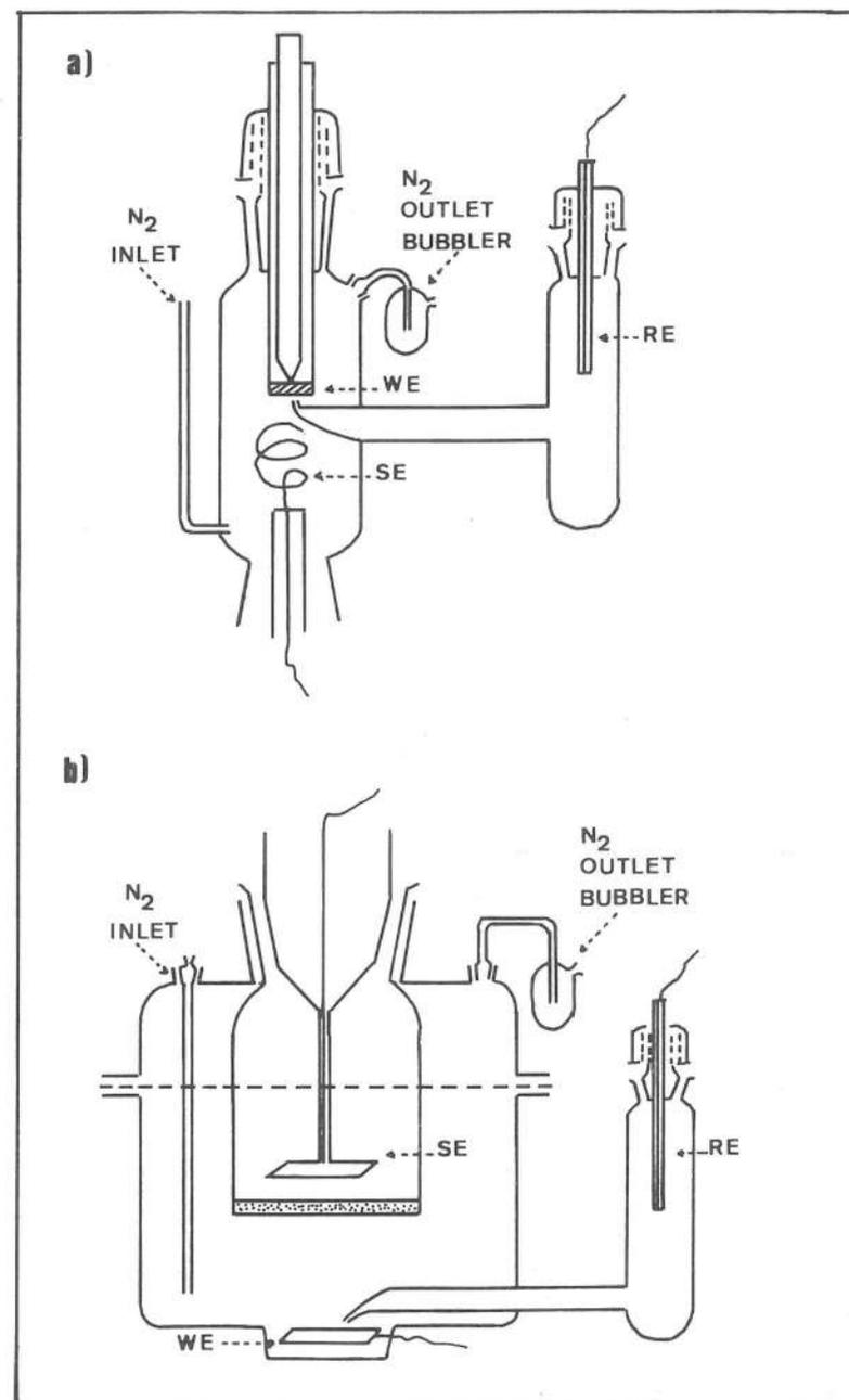
FIGURE 2 - Sketch of the cells used a) for cyclic voltammetry and b) for preparative electrolyses.
