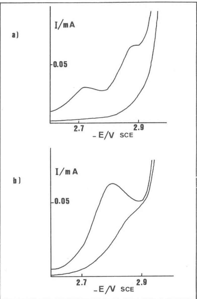
FIGURE 3 - a) Cyclic voltammogram for a solution of 0.005M Z-Leu<sub>2</sub>-OMe in 0.1M TBAB/DMF at a sweep rate of 0.1Vs<sup>-1</sup> at a vitreous carbon electrode of 0.05 cm<sup>2</sup> of area; b) Cyclic voltammogram for a solution of 0.005M Z-Pro-OBu<sup>t</sup> at the same conditions as in a).
