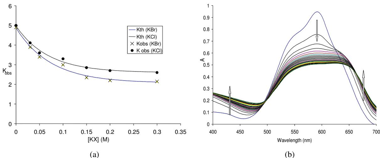
**Figure 5a.** Effect of halide salts on the discoloration rate constant (5 mL of  $12 \text{ mg L}^{-1}$  CV, 2 mL of  $0.05 \text{ M K}_2\text{S}_2\text{O}_8$ ,  $(3-x)$  mL of  $0.1 \text{ M KX} + x$  mL  $\text{H}_2\text{O}$ ). **5b.** Evolution of visible spectra during the discoloration of CV by persulfate in presence of  $2.510^{-4} \text{ M KI}$ . (Time of reaction: 20 min, scan every 40 s).
