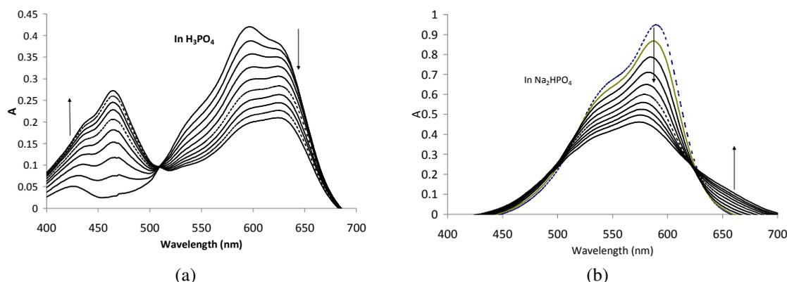
**Figure 4a, b:** Evolution of the visible spectra of the mixture CV and persulfate in  $\text{H}_3\text{PO}_4$  and  $\text{Na}_2\text{HPO}_4$  respectively. 5 mL of  $12 \text{ mgL}^{-1}$  CV, 2 mL of 0.05 M  $\text{K}_2\text{S}_2\text{O}_8$  and 3 mL of 0.1 M  $\text{H}_3\text{PO}_4$  and 3 mL of 0.1 M  $\text{Na}_2\text{HPO}_4$  respectively.
