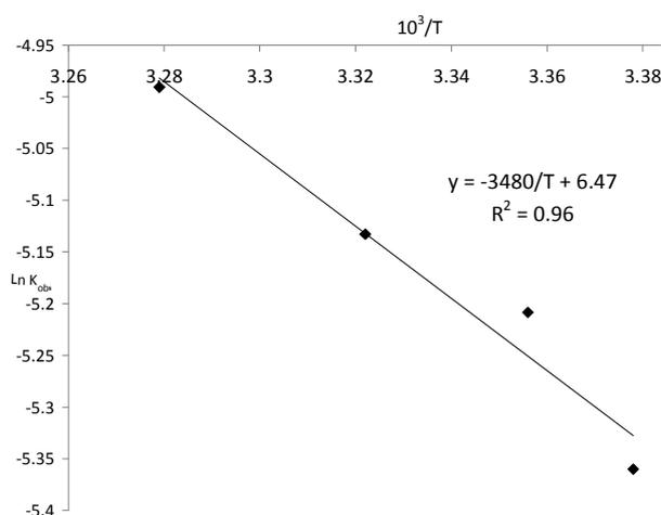
**Figure 8.** Arrhenius plot of  $\ln k_{obs}$  vs.  $1/T$ . ( $8.6 \text{ mg L}^{-1}$  CV ( $2.11 \times 10^{-5} \text{ M}$ ) +  $0.014 \text{ M}$   $K_2S_2O_8$ ).
