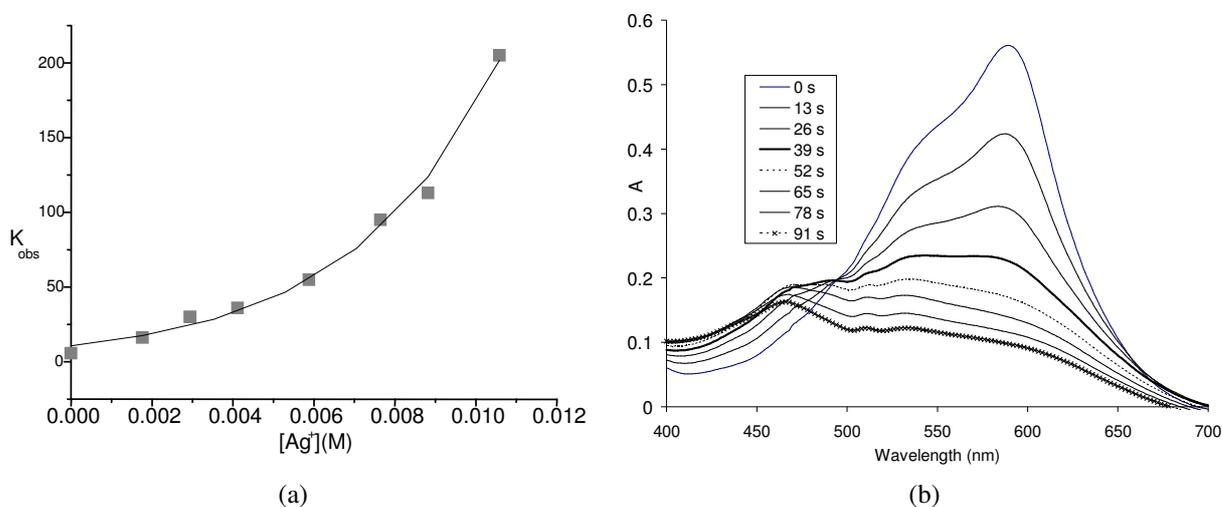
**Figure 6a.** Variation of the degradation rate constant of CV as a function of  $\text{Ag}^+$  concentration. 5 mL of 12 mg/L CV, 2 mL of 0.05 M  $\text{K}_2\text{S}_2\text{O}_8$ , (3- x) mL of 0.1 M  $\text{Ag}^+$  + x mL  $\text{H}_2\text{O}$ . **6b.** Evolution of CV spectrum during CV degradation with persulfate in presence of  $\text{Ag}^+$ .
