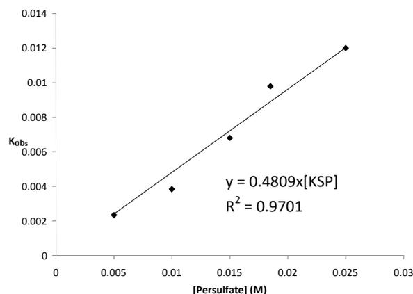
**Figure 3.** Pseudo order of the degradation of CV with respect to persulfate ( $k_{obs}$  in  $\text{mg}^{-1} \text{ L s}^{-1}$ ). (5 mL of  $12 \text{ mg L}^{-1}$  CV +  $(5 - x)$  mL of 0.05 M persulfate +  $x$  mL of 0.05 M of  $\text{Na}_2\text{SO}_4$  with  $1 < x < 5$ ).
