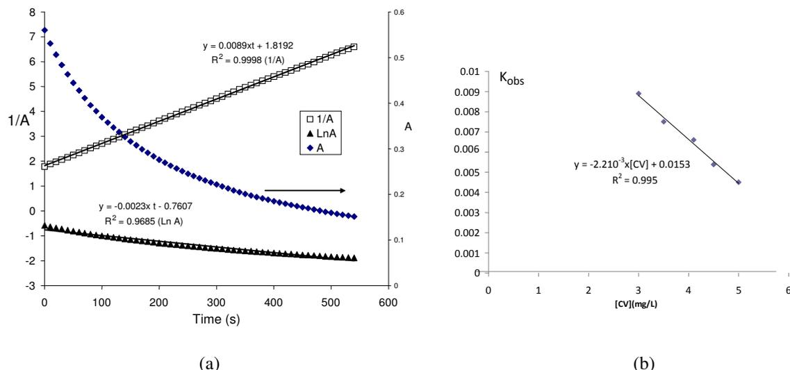
**Figure 2a.** Pseudo order of CV degradation with persulfate (A:Absorbance at 590 nm). (3 mL of  $12 \text{ mg L}^{-1}$  of CV + 5 mL of 0.05 M persulfate + 2 mL of  $\text{H}_2\text{O}$ ). **Figure 2b.** Effect of the initial CV concentration on the rate constant  $k_{obs}$  ( $\text{mg}^{-1} \text{ L s}^{-1}$ ).  $x$  mL of  $12 \text{ mg L}^{-1}$  of CV + 5 mL of 0.05 M persulfate and  $(5 - x)$  mL of  $\text{H}_2\text{O}$  ( $3 < x < 5$ ).
