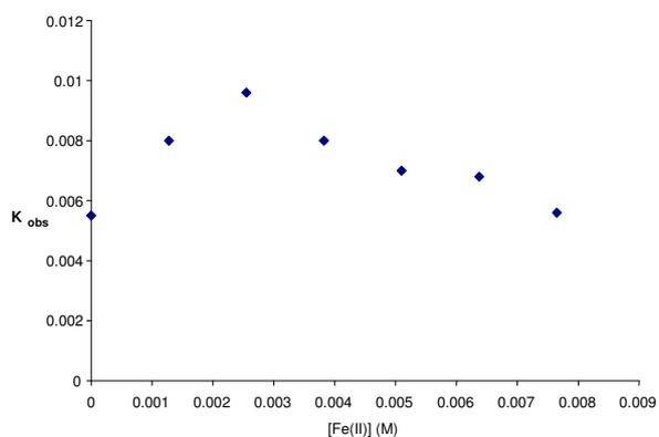
**Figure 7.** Variation of the degradation rate constant ( $k_{\text{obs}}$ ) of CV as a function of  $\text{Fe}(\text{II})$  concentration.
