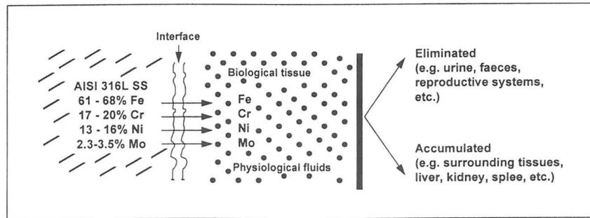
Figure 1 - Schematic representation of the AISI 316L stainless steel biodegradation process.
