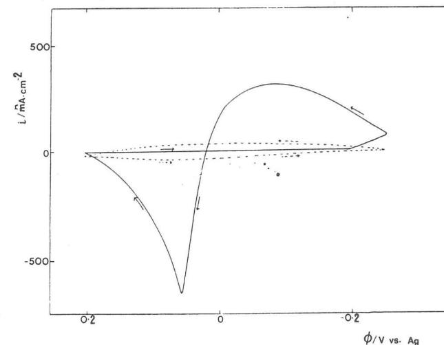
Figure 6 - Cyclic voltammogram for the deposition of silver onto vitreous carbon microelectrode ( $d = 5 \mu\text{m}$ ) from 5.0 mM  $\text{AgNO}_3$  in 0.1 M  $\text{KNO}_3$  aqueous solution (solid line) and only in 0.1 M  $\text{KNO}_3$  (broken line) at  $v = 100 \text{ mV/s}$ .
