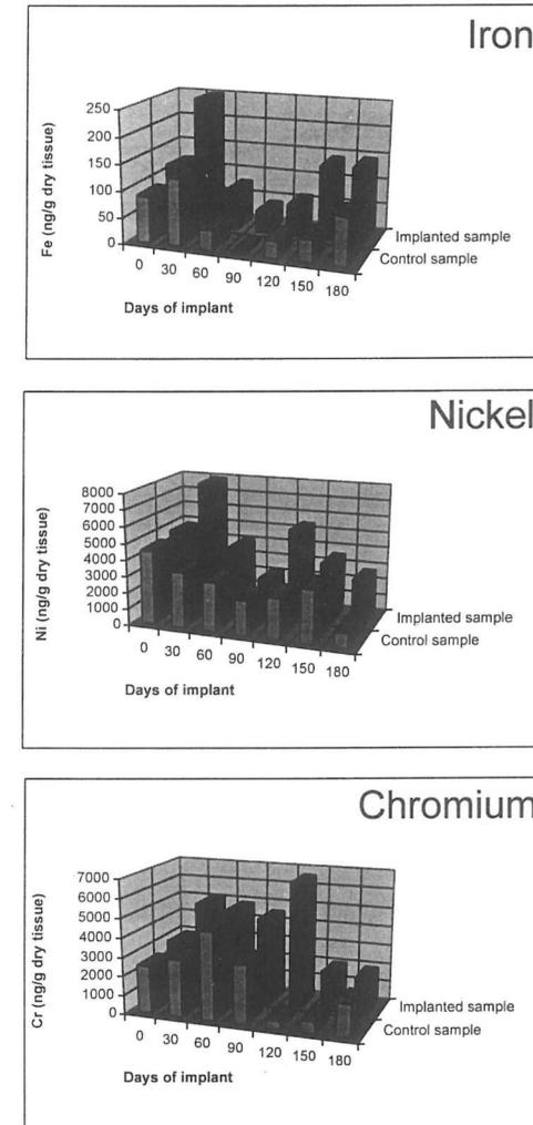
Figure 2 - Atomic absorption spectrometry analysis of biological tissues surrounding an AISI 316L stainless steel implant and control samples: (A) iron levels; (B) nickel levels; (C) chromium levels.
