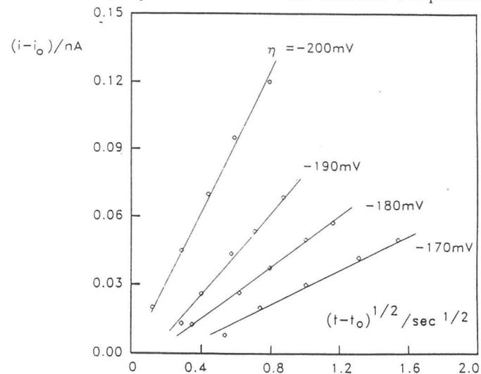
Figure 8 - Test of the kinetics of growth of Ag centers on carbon microelectrodes.
