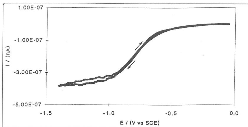
Figure 5 - Steady-state voltammogram of iron in a mouse spleen sample using a Au microelectrode (d = 25 μm) at v = 500 mV/s.
