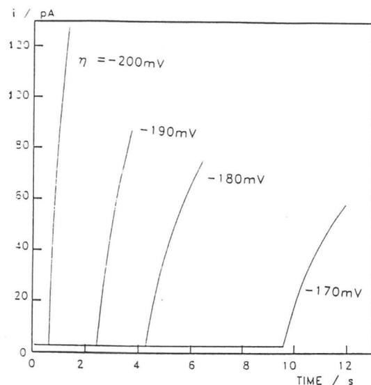
Figure 7 - Current-time transients for the growth of Ag on a vitreous carbon microelectrode ( $d = 5 \mu\text{m}$ ) from 5.0 mM  $\text{AgNO}_3$  in 0.1 M  $\text{KNO}_3$  aqueous solution at the indicated overpotentials.
