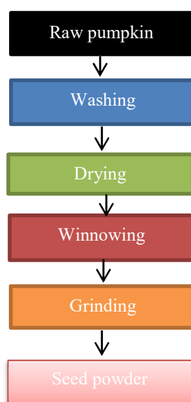
Figure 1: Flowchart for the preparation of PS powder.
