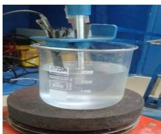
**Figure 10:** Conventional pyrex glass cell.
