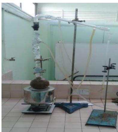
**Figure 7: Clevenger apparatus.**
