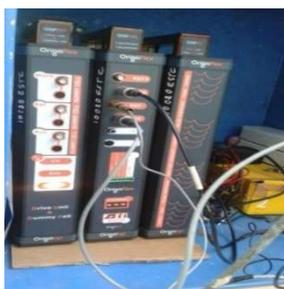
**Figure 11:** Origa Flex potentiostat.
