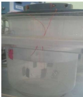
**Figure 12:** Al WL experiments in 500 mL of 3% NaCl.
