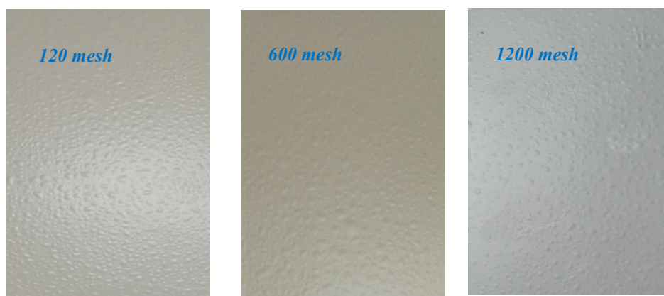
Figure 11: Salt spray test, with an IT of 15 days.
