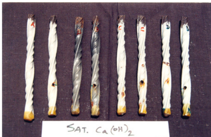
Figure 4. Photograph of coated rebars immersed in 3 M Ca(OH) 2 solution for a duration of 60 days.
