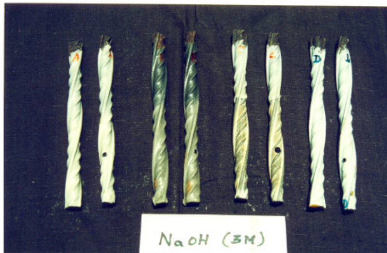
Figure 3. Photograph of coated rebars immersed in 3 M NaOH solution for a duration of 60 days.
