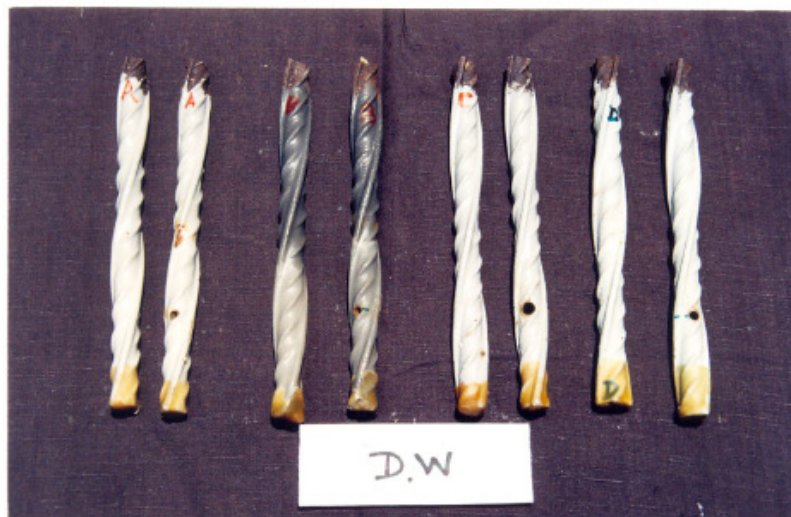
Figure 5. Photograph of coated rebars immersed in distilled water for a duration of 60 days.
