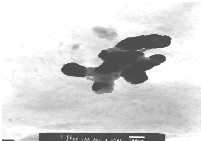
Figure 2. SEM micrograph (a), TEM micrograph (b) of a Pt-Ru-Pani electrode (EDX analysis 30 atom % Ru).
