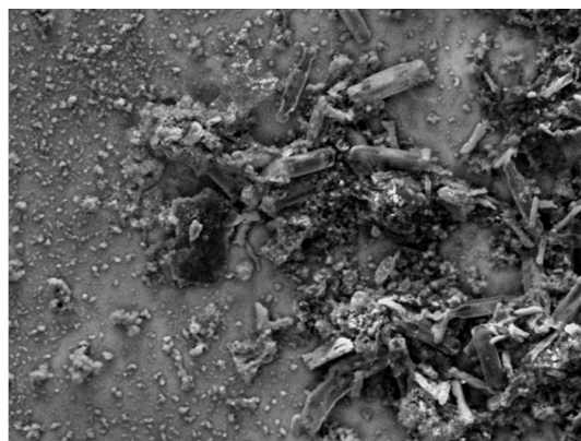
Figure 4. Photomicrograph taken by the scanning electron microscope, of inconel 600, incubated with culture B8 for 4 weeks, 100X.
