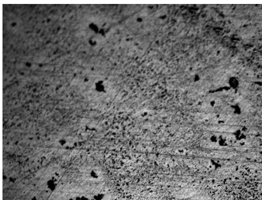
Figure 3. Photomicrograph taken by the scanning electron microscope, of inconel 600, incubated with culture B8 for 8 weeks, 100X.
