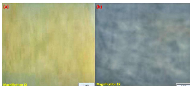
Figure 3: Photographs of samples CC - (a) chromate solution after 15 min of treatment in the chromate bath - (b) \text{MnO}_4^- solution after 24 h of treatment in \text{MnO}_4^- bath.
