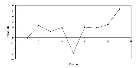
Figure 8. Residuals vs. run of hardness.
