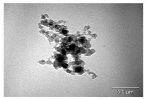
**Figure 3**. Transmission electron micrograph of 8 YSZ Tosoh powder.
