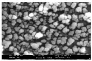
Figure 2. Scanning electron micrograph of 8YSZ powder (Tosoh).
