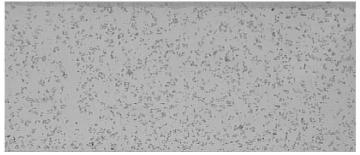
Figure 4. Cross-sectional optical micrograph of Ni-YSZ coating.
